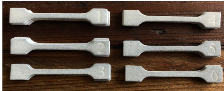
Figure 8: Completed 3D Printed Dogbone Samples
