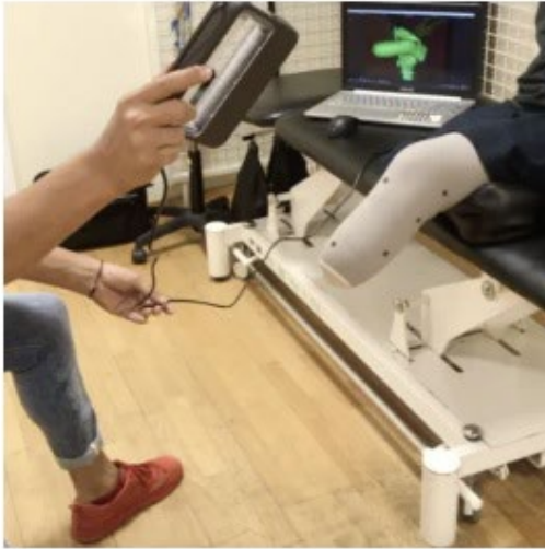
1: Your prosthetist scans your limb at the clinic to produce a basic 3D image. Elapsed time: a few minutes.
