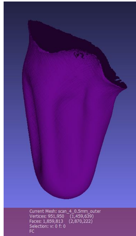
Figure 6: 3D scan of outer surface of inner socket (0.5 mm resolution)
