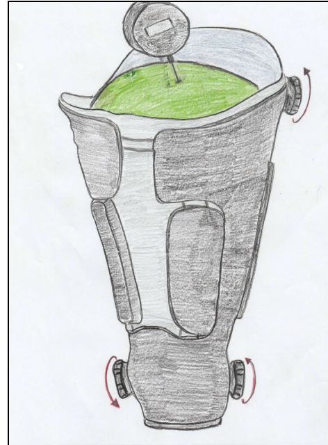
Figure 8: Volumetric testing set up with the air bladder inside the Quatro socket. Arrows indicate the direction at which the dials were turned.
