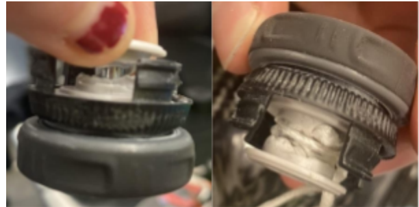
Figure 17: Failure of BOA dial at center plastic spool from volume testing.
